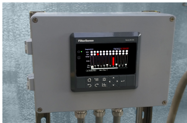
B-PAC ultra-rugged (field-mountable) user interface displays diagnostics (data also available over Fieldbus).
