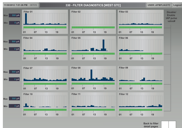
Control Room view of DynaCHARGE leak detection by row.
